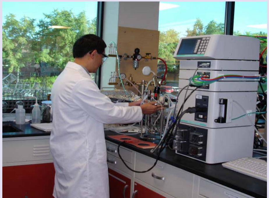
Dr. Haixuan Zou of The Pulp & Paper Process Development Center conducts testing using a bioreactor for a bio-refinery experiment.
