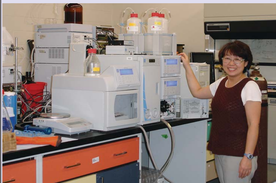
Seongkyung Park, Analytical Chemist, UMaine Process Development Center, performing testing on the HPLC.
