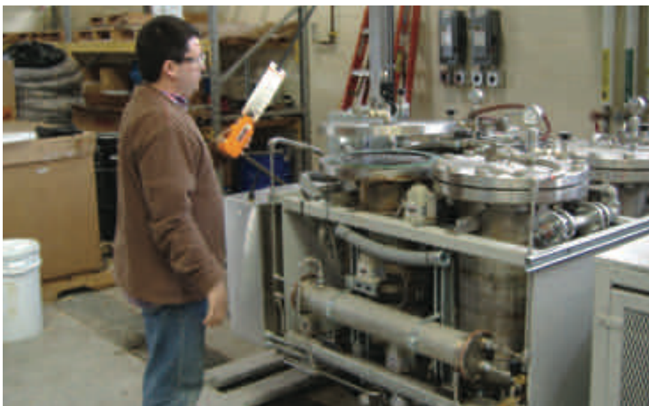
Juan Peredes, UMaine PhD Candidate extracting hemi-cellulose from southern yellow pine strands to improve the strength of OSB.
